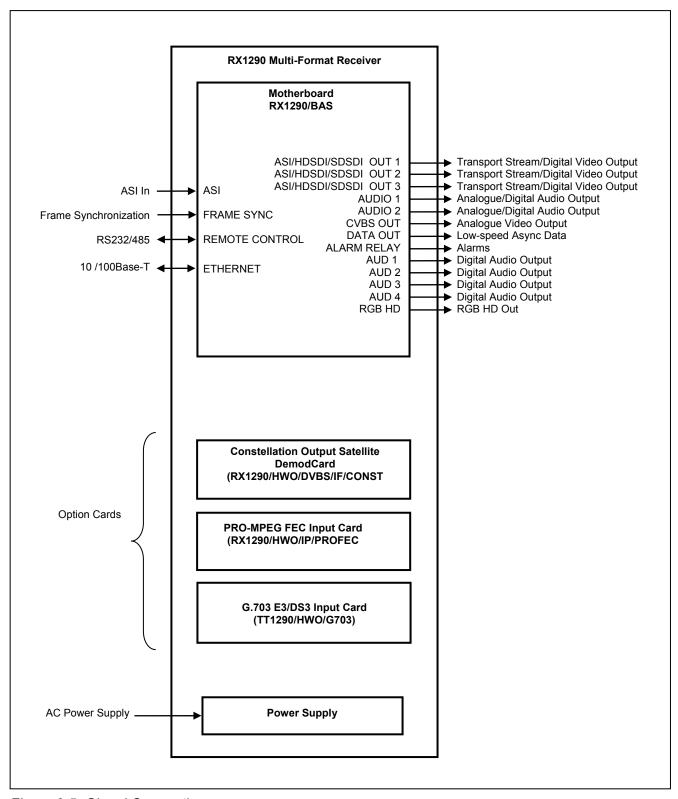
Figure 2.5 Signal Connections
